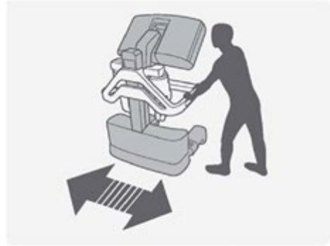
Label on Surgeon Console: Move Surgeon Console using handles on side
