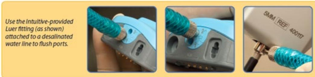
Use the Intuitive-provided Luer fitting (as shown) attached to a desalinated water line to flush ports.
